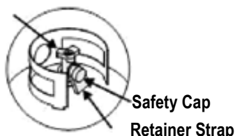
LP Tank Valve
